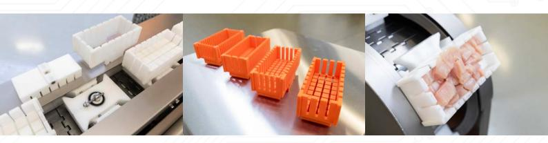
Another unique feature on the MATRIX is that IFEC can supply the cutting molds easily according your specifications. With using the most modern 3D printing techniques IFEC can easily make prototypes.
