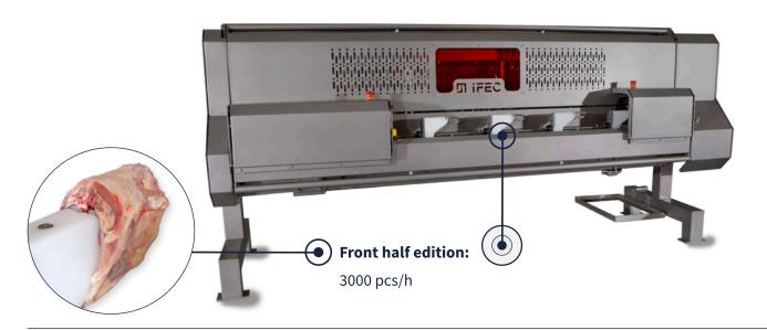
The back meat harvester front half edition has a capacity of 3000 pieces per hour. The front half carcasses are manually loaded onto specially designed cones, outfitted with a locking mechanism that ensures perfect alignment. Due to an extra pre-cut module, the back meat and remaining carcasses are automatically separated and unloaded. The final product is a beautiful piece of back meat
