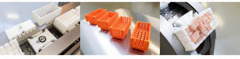
Another unique feature on the MATRIX is that IFEC can supply the cutting molds easily according your specifications. With using the most modern 3D printing techniques IFEC can easily make prototypes.
