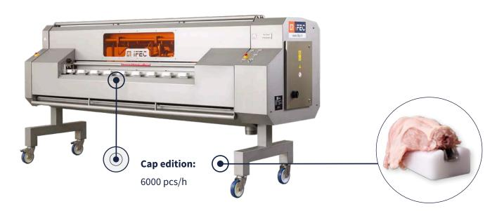
The back meat harvester caps edition has a capacity of 6000 pieces per hour. The upper backs are manually loaded onto specially designed cones. The back meat and remaining upper backs are automatically separated and unloaded. The final product is a beautiful piece of back meat suitable for further processing. Optionally, the back meat, including scapula bones, can be split into two pieces to transform it into a one-hand BBQ snack.
