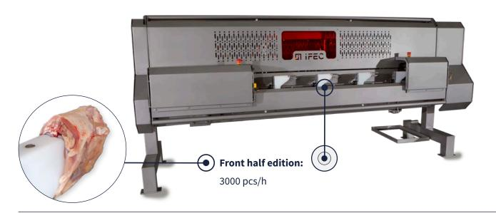
The back meat harvester front half edition has a capacity of 3000 pieces per hour. The front half carcasses are manually loaded onto specially designed cones, outfitted with a locking mechanism that ensures perfect alignment. Due to an extra pre-cut module, the back meat and remaining carcasses are automatically separated and unloaded.
